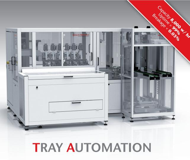
The Jonas & Redmann Tray Automation is a highly developed modular machine platform designed for the loading and unloading of process equipment based on an in-line concept, where the wafer transport is effected by flat carriers or trays. In addition to a wide range of options, this machine platform offers a series of innovations that serve outstanding wafer positioning accuracy, the reduction of wafer breakage and the uncompromising gentle handling to protect thin films.
